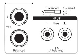
**Line-level Inputs.** The Eris E3.5 active monitor provides a choice of two pairs of inputs: left and right balanced ¼"TRS and left and right unbalanced RCA. These inputs accept a line-level signal from an audio source and feed that signal to the each monitor's built-in power amplifier. These inputs are provided to enable flexible connectivity, not for connecting multiple sources to your speakers simultaneously.
