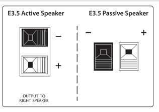
**Bare-wire connectors.** This connection is used to power and send signal to the passive E3.5. Be sure to connect the positive and negative connections on your active E3.5 to the positive and negative connections, respectively, on the passive E3.5 (i.e. connect positive to positive and negative to negative).
